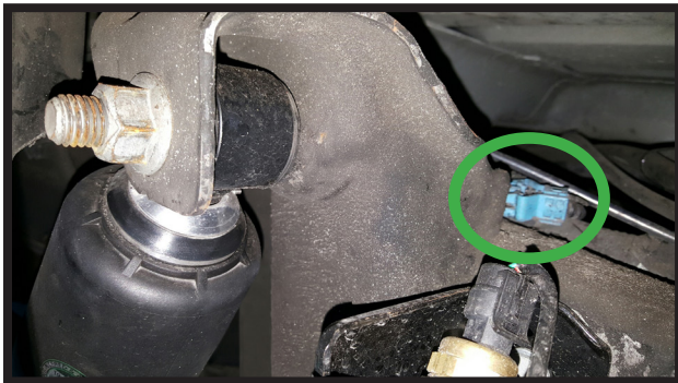
ABS Wiring Harness
